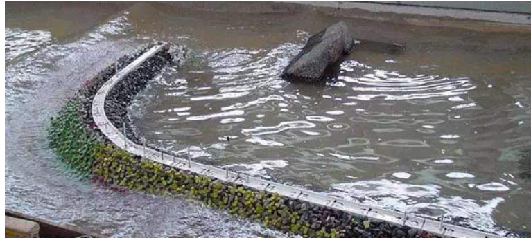
Figure 4 - Establishment of Physical Hydraulic Model
